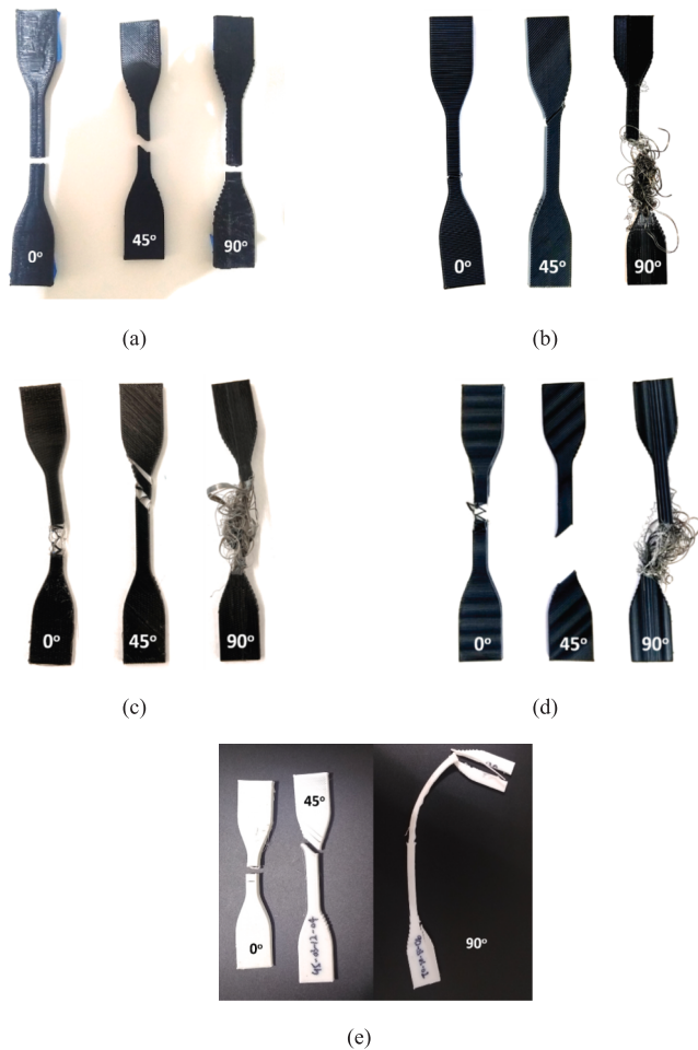
Fig. 20. 0°, 45°, 90° raster angle dogbone specimens ((a): PLA, (b): PLA:TPU = 60:40 in parallel, (c): PLA:TPU = 40:60 in parallel, (d): PLA:TPU = 40:60 in series, (e): TPU) after failure.
