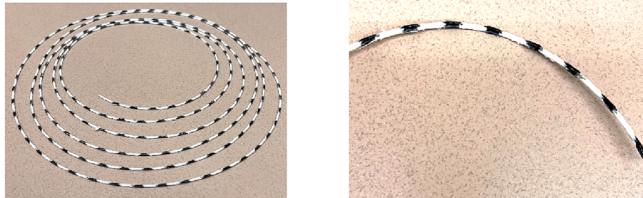
Fig. 5. Programmable Filament with a series configuration of PLA (black) and TPU (white).
