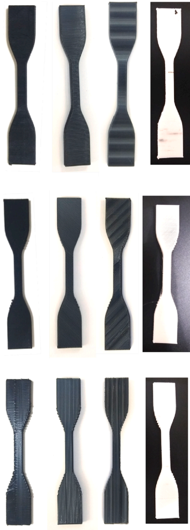
Fig. 10. Dogbone specimens (PLA – PLA:TPU 40:60 Parallel – PLA:TPU 40:60 Series – TPU) with raster angles 0^\circ (top), 45^\circ (middle), and 90^\circ (bottom).
