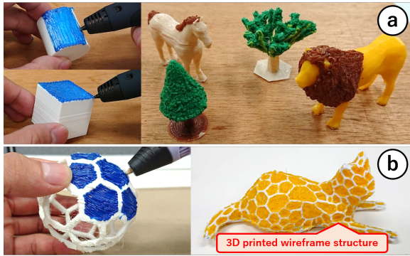
Figure 3: 3D doodling on 3D printed objects. (a) Users can produce works by stroking the surface or (b) filling wireframe structures using a 3D pen.
