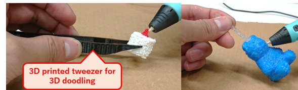
Figure 6: 3D doodling with 3D printed on-demand tools.
