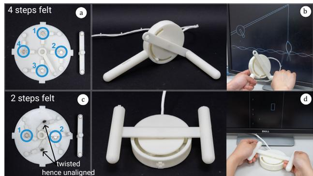
**Figure 13: The fishing rod mechanism has four steps of discrete feedback (a) felt when reeling-in fish in complete rotations. Reconfiguration changes the number of steps to two (c), felt during steering the controller to the left or right (d).**
