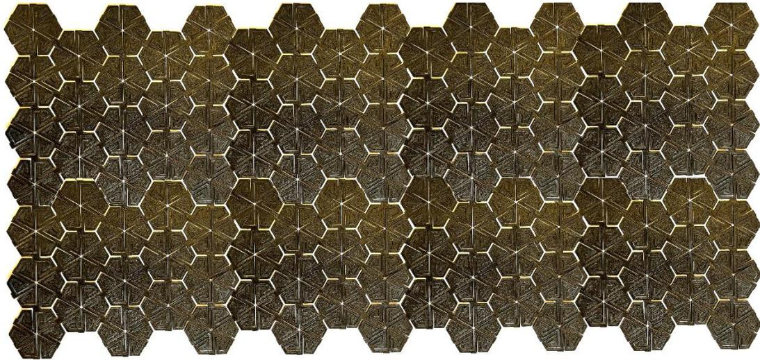
Figure 8. 3D printed PLA hexagonal kerf panel
