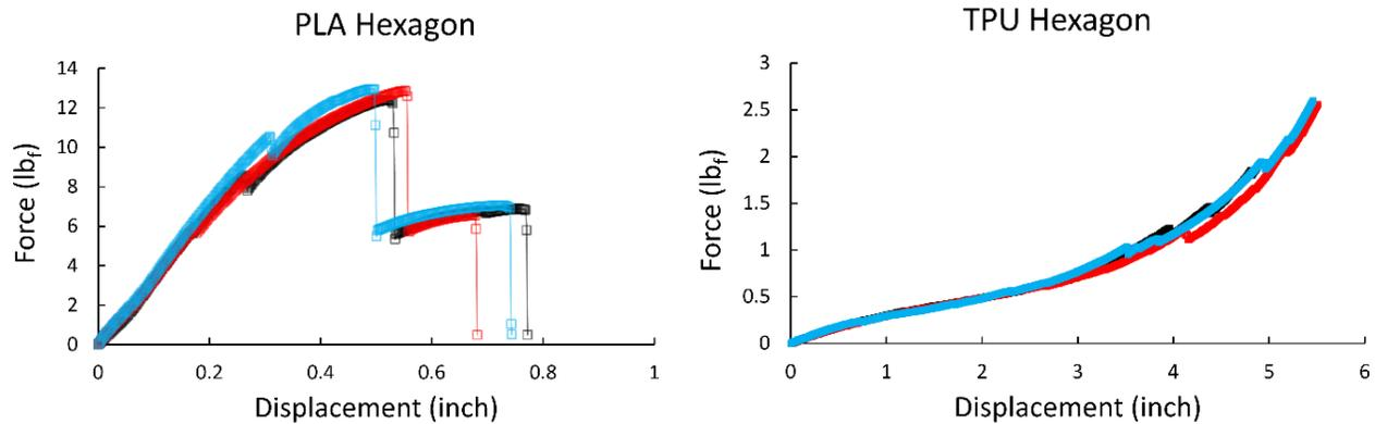
Figure 6. Force - Displacement curves for PLA and TPU hexagonal kerf unit cells
