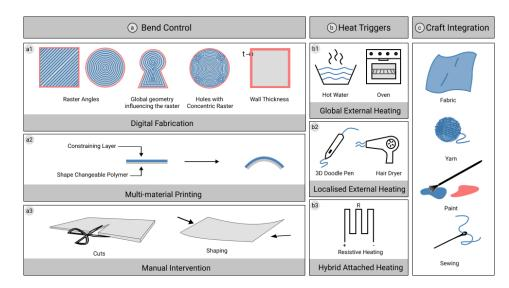
Figure 4: Fab4D Design Space: (a) Bend Control techniques include Digital Fabrication techniques, Multi-material Printing, and Manual Intervention, (b) Heat triggering techniques include Global External Heating, Localised External Heating, and Hybrid Attached Heating, and (c) Craft Integration includes combining external craft material with the printed artifacts
