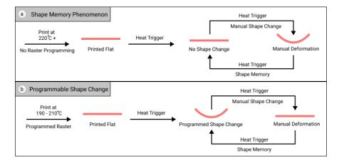
Figure 2: 4D Behavior of Thermoplastic upon heat trigger: (a) Shape Memory Phenomenon (b) Programmable Shape Change
