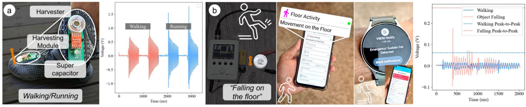
Fig. 11. A VIB3D module mounted (a) on a shoe harvests step-generated energy, increasing from walking to running, and (b) on the floor distinguishes walking (low-voltage) from falls (voltage spike).
