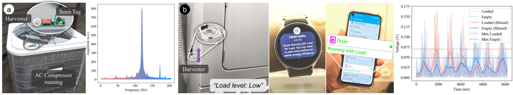
Fig. 14. A VIB3D harvester mounted (a) on an AC compressor captures operational vibrations, accumulates energy, and transmits Sozu beacons [53], with the vibration spectrum revealing characteristic frequency; and (b) on a dryer captures vibrations to distinguish loaded and unloaded states from signal energy.
