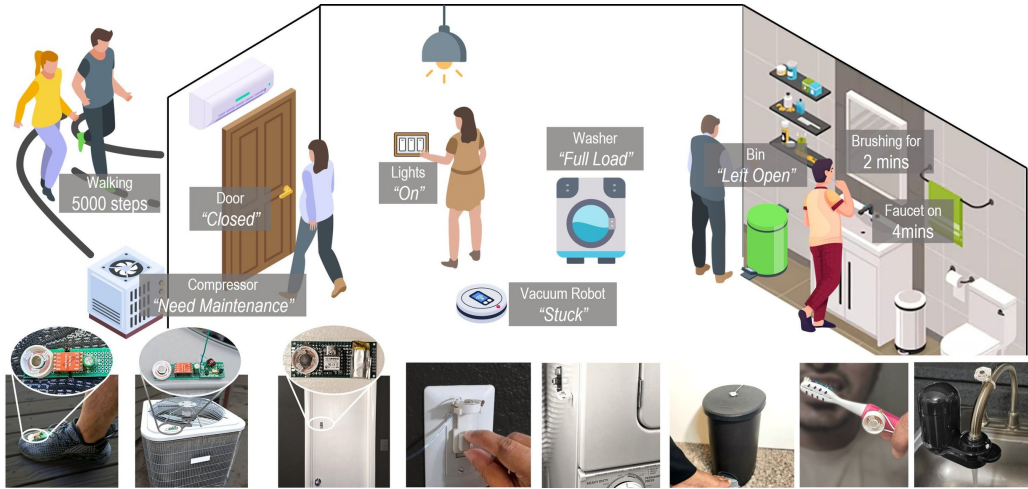
Fig. 1. VIB3D is a low-cost FDM-printed, self-powered, miniaturized vibration sensor for capturing everyday interactions and contextual signals, from workout quality and compressor performance to unique material identification and personal hygiene logging.
