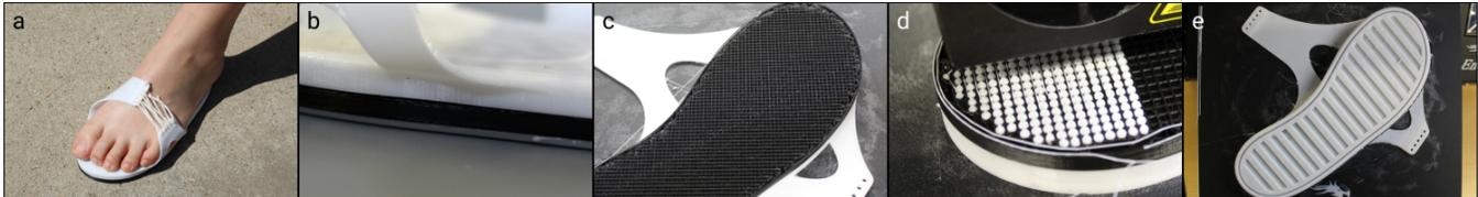
Figure 19: (a) Flip-flop in use, (b) a close up of the material change of TPU(white)-PLA(black)-TPU(white), (c)-(e) process of creating the lattice structure: starting with the buckets, material purged into buckets, then covering with the final layer.
