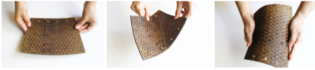
Figure 2: Kerf structures are often the results of subtractive fabrication, imparting flexibility to rigid sheets.
