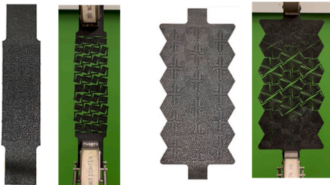
Fig. 15. Experimental setup for square and hexagon kerf structures under uniaxial tension.
